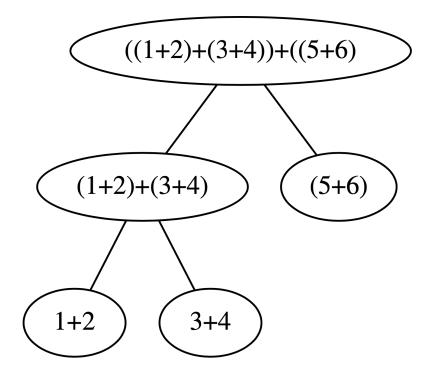
Each circle is a *node* of the tree.<sup>1</sup> The *work*, W, of the expression tree is the total number of nodes, while the *span*, S, is the number of nodes along the longest path from the top to the bottom.
